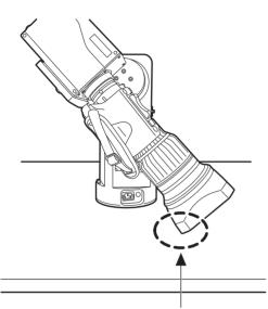
Lens must not come into contact with mounting surface.
